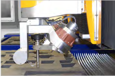
Intelligent taper compensation for true contour edges
