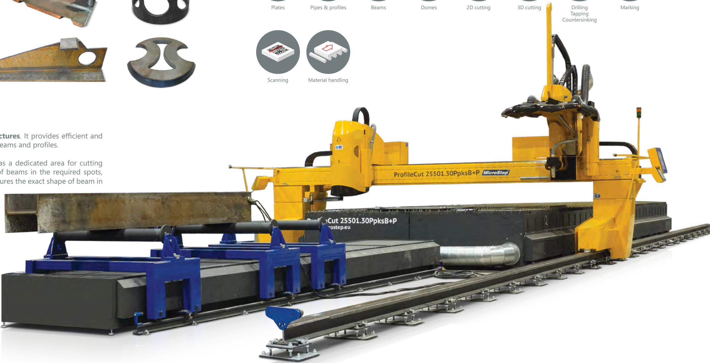
Great production flexibility thanks to the 120° bevel cutting head
