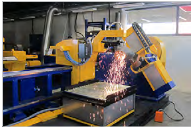
ElbowCut: Weld edge preparation on pipe elbows
