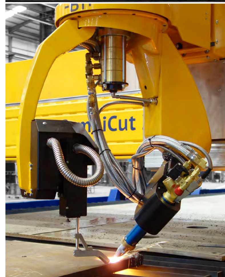
Bevel cutting with oxyfuel rotator
