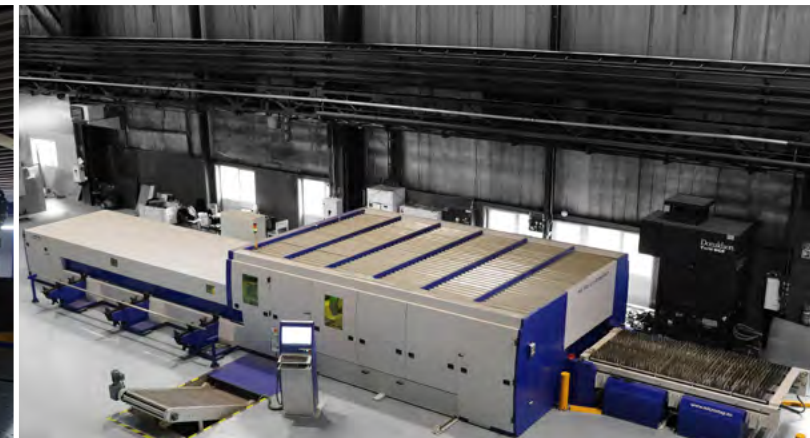
A combined machine with automated pipe cutting
