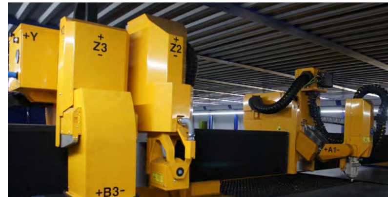
Multi-functional machine with additional beveling and inkjet marking
